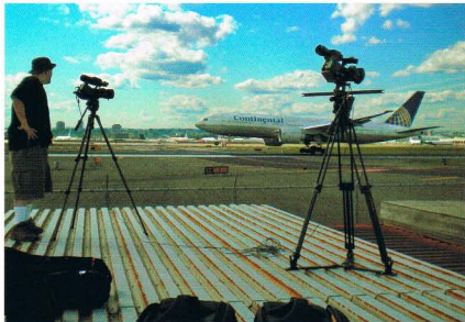
Filmmaker Jerome Bongiorno operates two linked Sony XDCAM EX3s set up for a hyperstereo shot of a plane landing at Newark airport on a windy day.
