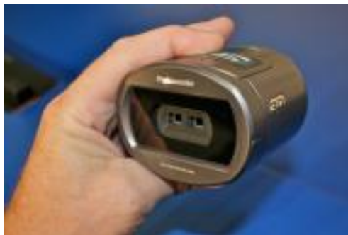
Innovative 3D lens module that converts HDC-SDT750 camcorder body to stereoscopic mode.
